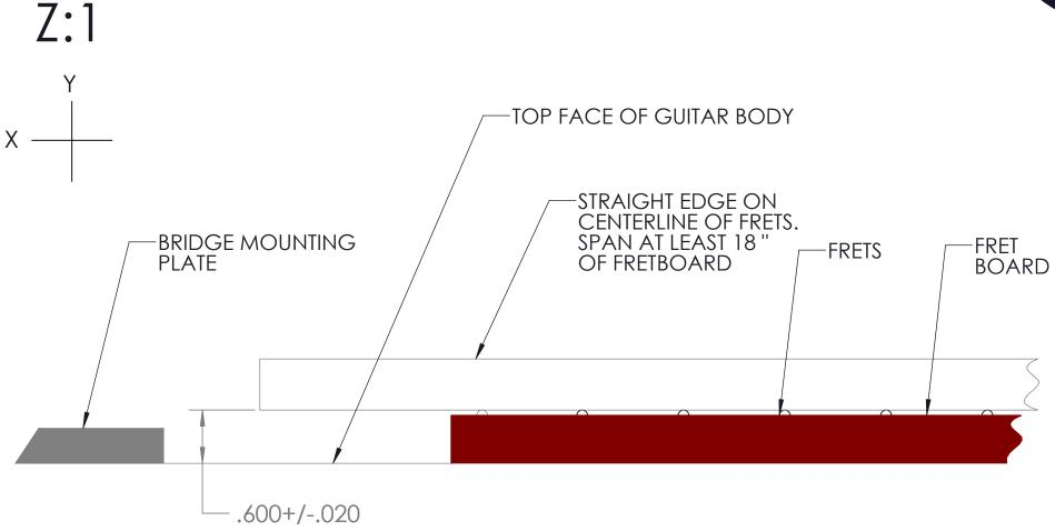
NOMINAL HEIGHT. IF GREATER, ADJUST NECK ANGLE OR ADD SHIMS UNDER BRIDGE PLATE. IF LESS, ADJUST NECK ANGLE OR ROUTE AN INSET.
